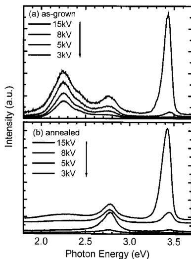
FIG. 2. CL spectra with four different electron voltage levels for the samples before (a) and after (b) thermal annealing.
