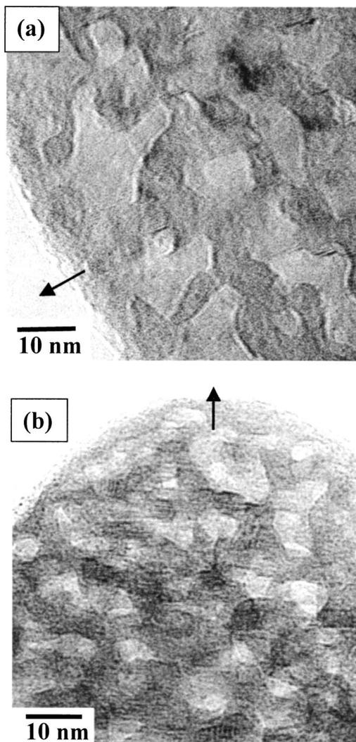
FIG. 5. Typical HRTEM images before (a) and after (b) thermal annealing. Arrows show crystal growth directions.
