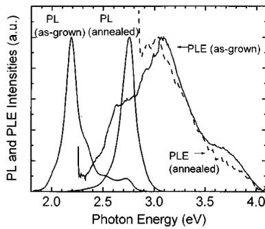
FIG. 1. PL and PLE spectra at 10 K before and after thermal annealing.
