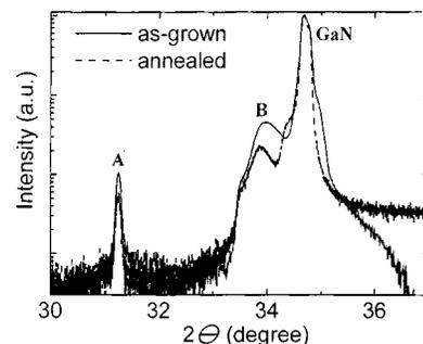
FIG. 4. XRD patterns before and after thermal annealing.
