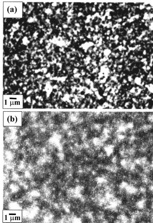
FIG. 3. (a) Typical CL image before thermal annealing; (b) typical CL image after thermal annealing.
